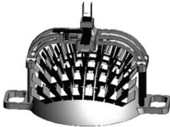
7x8 sensor fixture With ceramic strips + heat sinks
